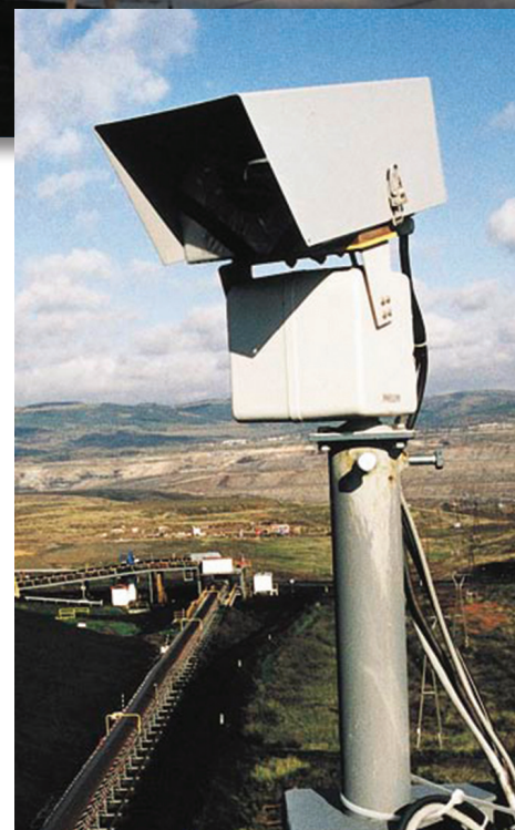
The FLIR Systems thermal imaging camera mounted on a mast over the coal piles of the Nástup Mines Cooperation in the Czech Republic.
