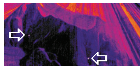
The overlay of a coal pile with 2 hot spots as possible combustion points.
